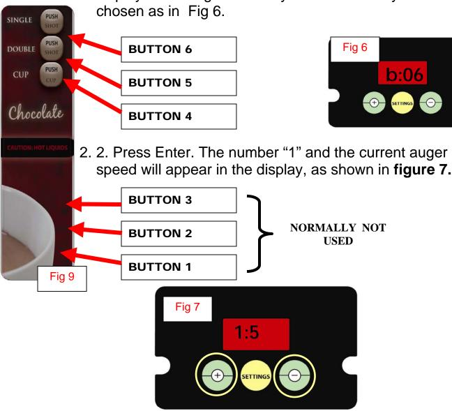
3. Using the + or – button to scroll, set Auger speed for the desired speed.
