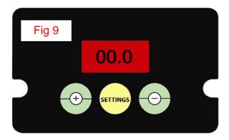
5. Press and release the "settings button to store switch settings. The display will return to "SEL". To program another switch, repeat the instructions for programming the selector switch, above. Pressing the settings button after all the switches have been programmed will return normal operating mode and the display will change to "--" as in figure 1, above.
